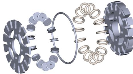
*Fig. 2: Exploded view of an omniwheel.*
