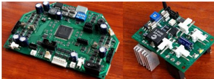
Fig. 2. Robot's controller, Left: Main electronic board, Right: Kicker board
