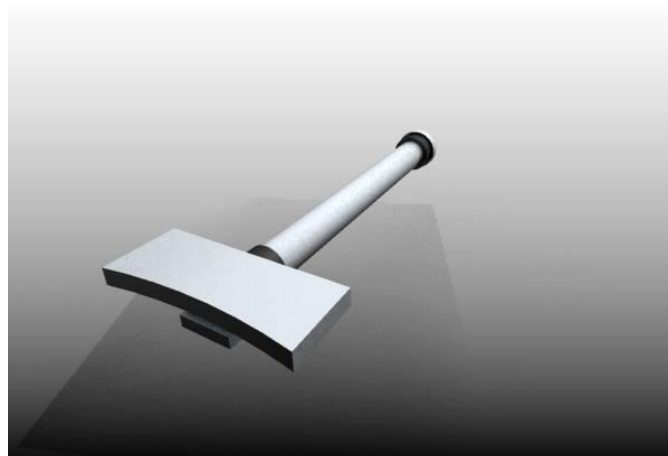
Figure 9: 3D Design of Kicker with Rubber Washers at both ends.
