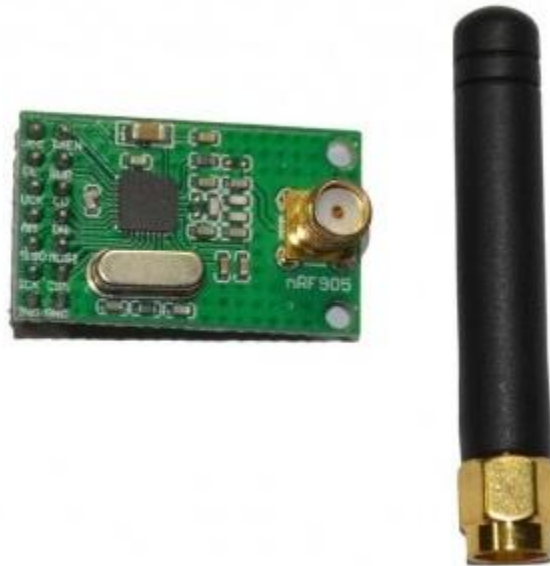
Figure 3: Image of NRF905 Wireless Module [1].
