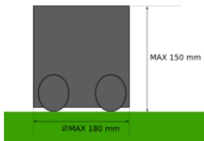
Figure 3: The maximum robot dimensions
