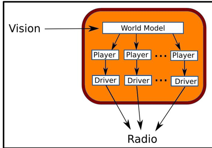
Fig. 5. GEAR AI architecture
