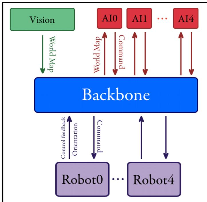
Fig. 1. GEAR System architecture
